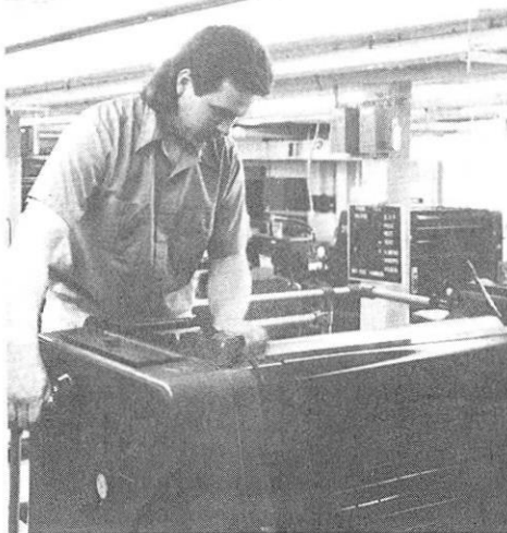
DoD student Richard Vickers cleans the ink fountain roller on the Heidelberg SORD printing press.
