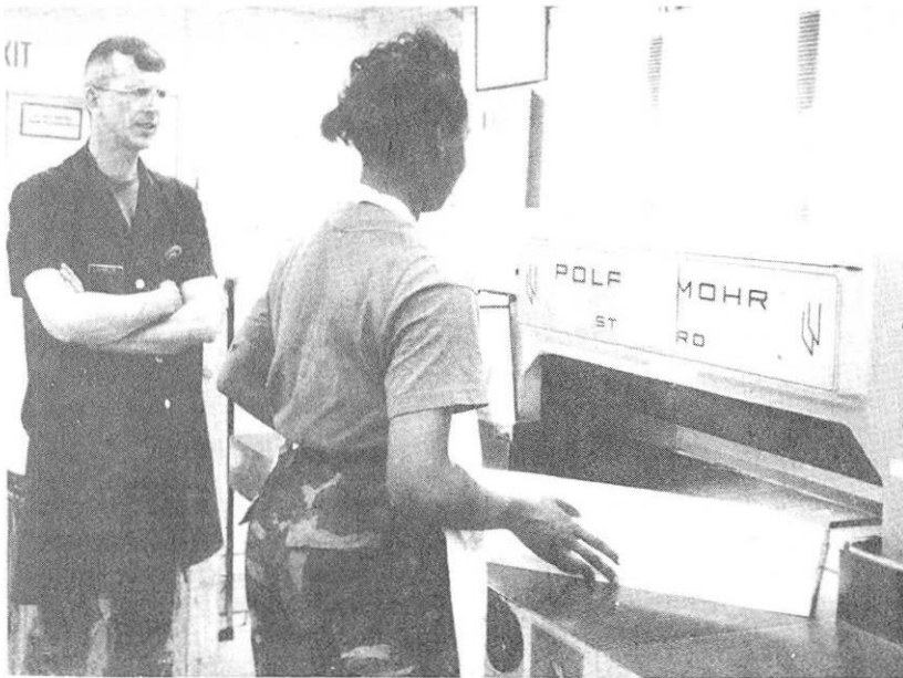
Senior Instructor SSgt Michael Hamblen watches carefully as BOP student positions paper in hydraulic paper cutter.
