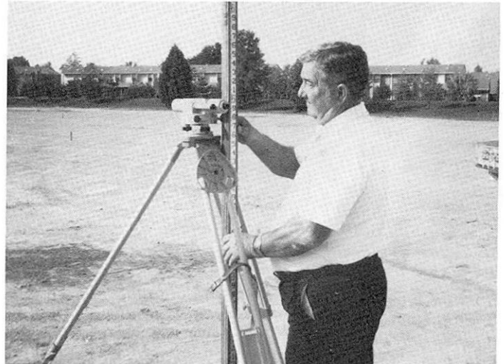
Andy Bradley measures the height of instrument, which is needed to determine elevation. (Photo by SSgt D. K. Jones)
