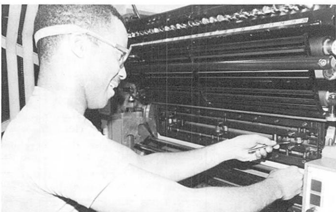
SGT Morgan tightens the tail clamp tension nut on the plate cylinder to secure the plate around cylinder.
