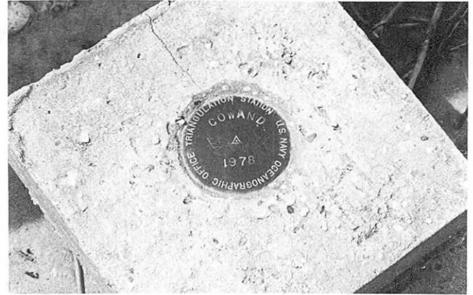
A triangulation station installed in the Bay St. Louis area by HYCOOP instructors, for student use in practical exercises.
