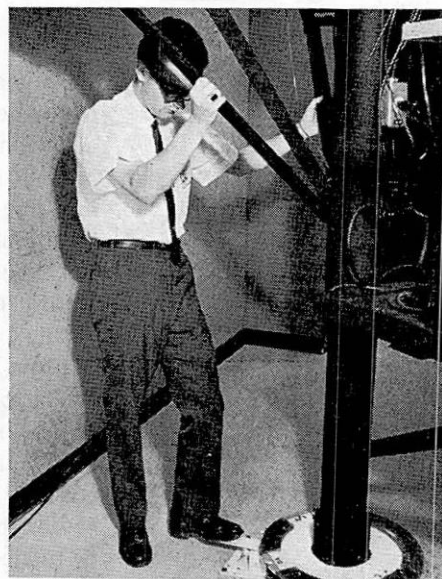
He presses brake pedal, and rotates tree until right projector clicks into place.
