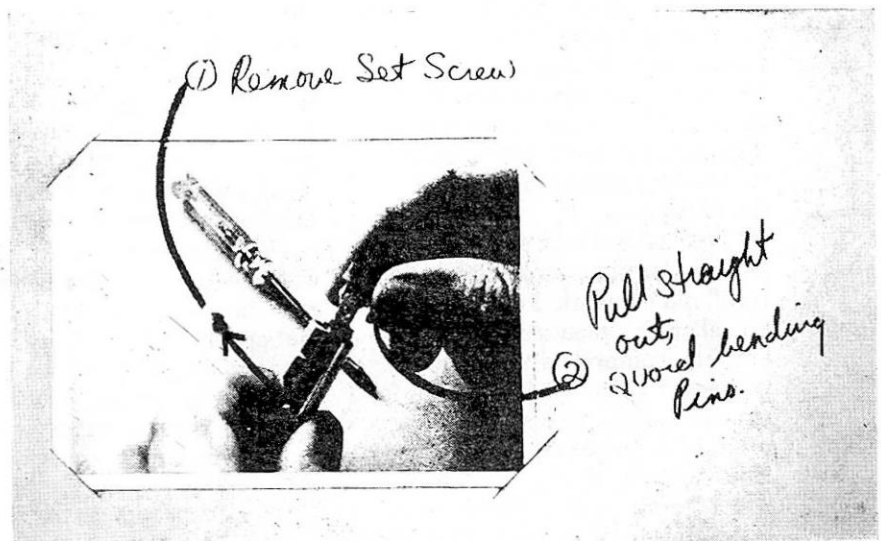
Final system of photos and handwritten instructions followed when foremen showed reluctance to scrawl changes over neat typewriting.
